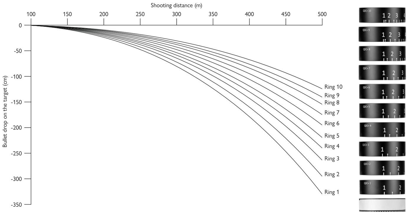
The ballistics calculator tells you the appropriate ring and provides a clear illustration of the trajectory.
