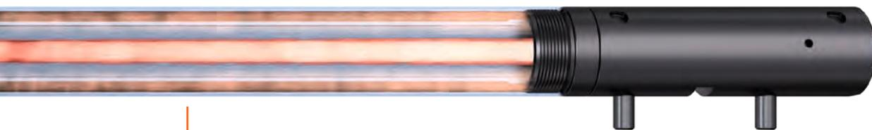
The innovative design of the Blaser Integral Silencer allows for use of the entire length of the silencer as an expansion space for the powder gases – while maintaining its slim overall appearance. The inner tube of the Blaser Integral Silencer (ISD) contains and closes off the expansion chamber and keeps the gases from contacting the surface of the barrel itself. The barrel always remains clean and is reliably protected against powder residues, contamination and corrosive residues.
