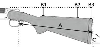
**A** = Stock lengths (measured with trigger in middle position)
